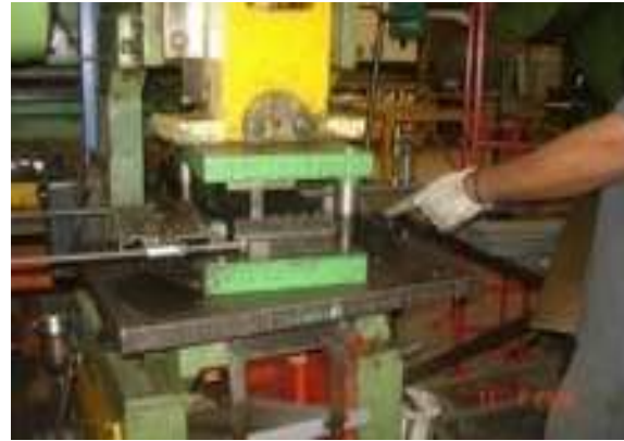
Press tool for strip(W-300) parting
