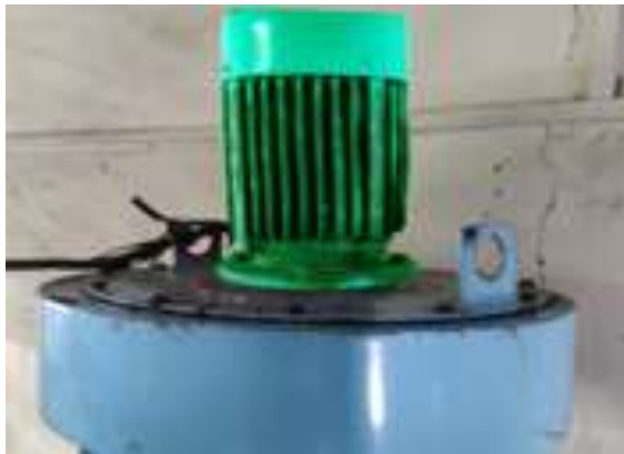
Powder Recovery Blower Motor (3 HP )
